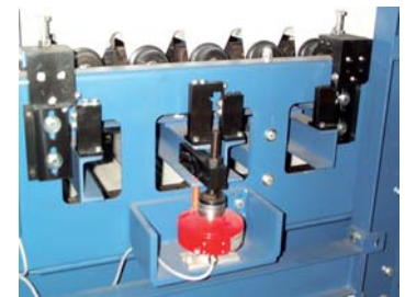
Weighbridge Digital load cell
